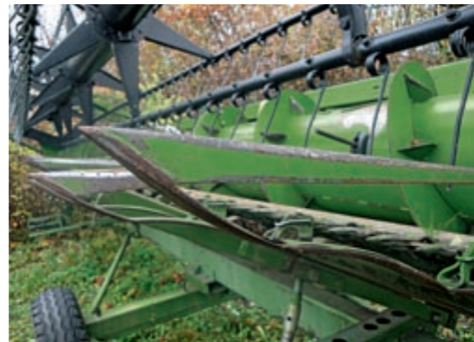
Crop lifter inspection. Check crop lifters to see if any are bent or damaged. Bent crop lifters will reduce the performance of the combine. If they are bent downwards, they could even damage the header by digging into the ground.
