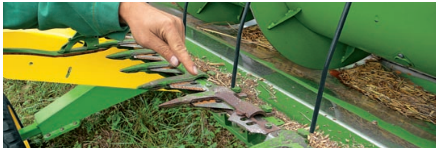
Knife and section guards inspection. Check to see if any of the knives or the knife guards are broken or bent and replace where necessary. When replacing a knife, be sure to use genuine John Deere knife sections to ensure that the knife has the durability and the size needed for optimal operation.
