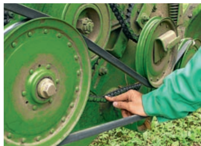
Adjust drive parts. The cutting belt drive and the auger chain drive can be adjusted on the right side. Remove the left hand side shield and check tension of belt and chain to ensure optimal header performance. See operator's manual for optimal adjustment.
