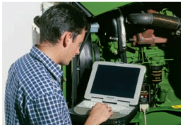
For late-model John Deere equipment, our technicians use the Service ADVISOR diagnostic tool. Linked directly to your machine's electronic controllers, this valuable tool enables our service technicians to determine problems faster and more accurately than ever before.
