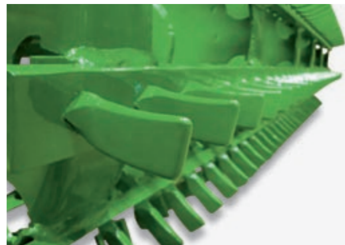
Spike tooth cylinder and concave. Specially designed to deal with the difficulties of threshing rice, this bundle contains a cylinder and a concave which are both equipped with teeth. These teeth provide very soft treatment of the rice, preventing damage to the rice corn and making your rice harvest much more efficient. In tough conditions with green straw it prevents concave plugging. Part No. BZ100225/BZ100226
