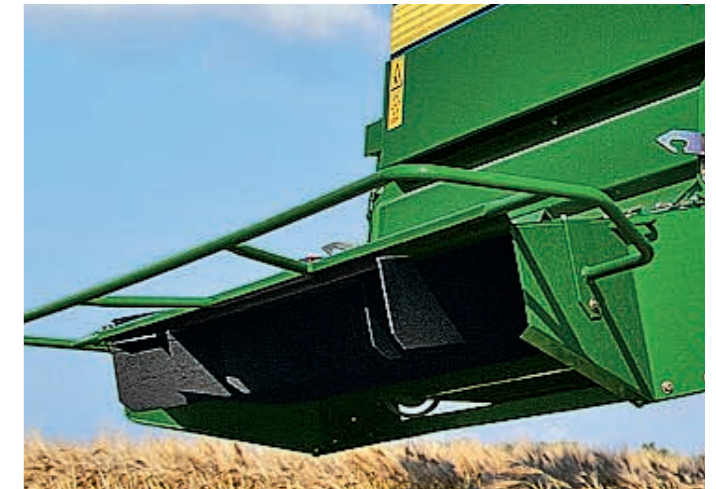
Premium chopper rebuild kit. Transform your standard straw chopper into a premium straw chopper. With an increased number of knives, this kit allows greater throughput with consistently high chopping quality. The kit includes a tailboard and should be used in combination with the premium chaff spreader. Part No. BZ13498/BZ13499/BZ100105/BZ100106
