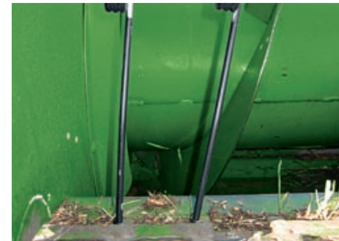
Check the reel tines. Check the reel tines to ensure that none are bent or damaged. Replace where necessary.
