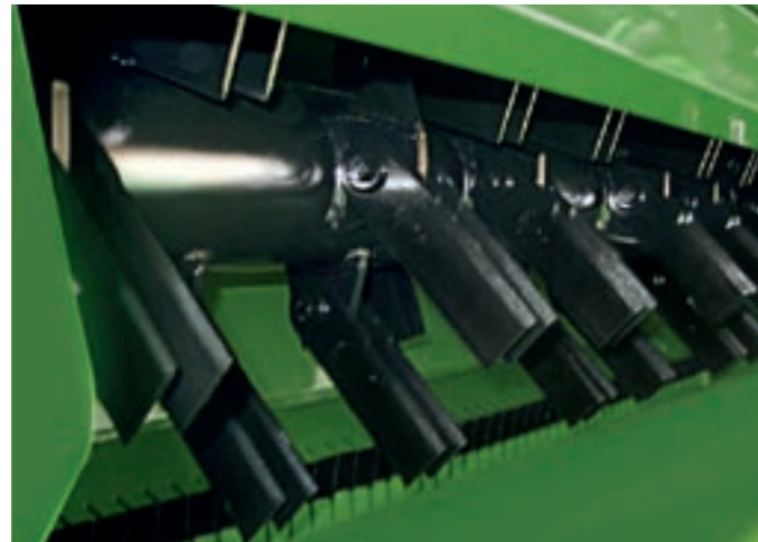
Standard chopper. Standard straw chopper with 3600 rpm rotor speed. Provides a very regular, fine cut. Drive parts are included. Part No. BZ13415/13416
