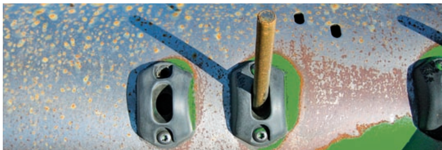
Auger finger inspection. Check to see that no auger fingers are broken or bent. Genuine John Deere auger fingers feature a breakaway groove, permitting them to break at a specific point and fall back into the auger drum to prevent platform damage.
