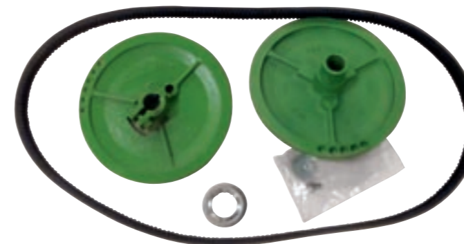
Slow fan speed. By reducing the fan speed from 650 to 350 rpm you can allow light crops to fall through the sieves instead of being blown out of the machine. Part No. BZ13666
