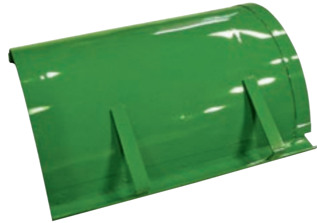
Top covers for C-series rotors. Reduce separator losses by installing a set of 10° top covers (1 x left hand, 1 x right hand cover) in middle position rather than the standard 20° covers. The two 10° top covers allow you to keep the material in the machine for a longer time, resulting in a more efficient separation process. Part No. AH13677 (left) / AH13678 (right)
