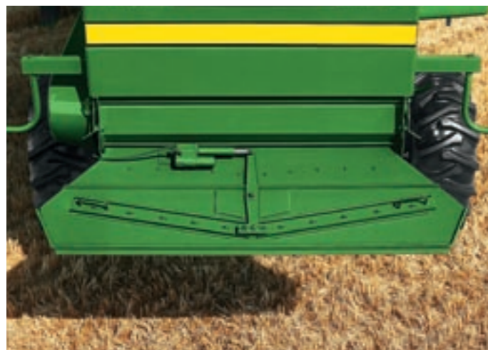
Tailboard with electric remote control. Designed for use with a standard chopper, this tailboard has an electric remote control making it easy to adjust the chopper vanes on-the-go when harvesting under difficult conditions (side wind). Part No. BZ13395/BZ13398
