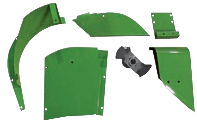
Grass kit for clean grain elevator top housing. Propeller turns in same rpm as filling auger to prevent a build-up in the transition area between the elevator and the filling auger. Part No. BZ100040/BZ100233
