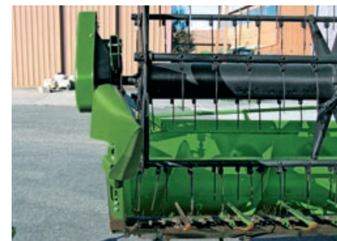
Crop divider inspection. Check crop dividers to see if they are damaged or bent. Check hinges to see if the crop dividers move properly. Bent crop dividers result in higher header losses and lower combine performance.
