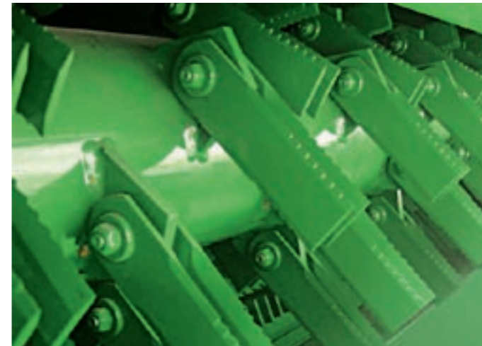
Premium chopper (2). The premium straw chopper with 3500 / 1700 (for corn) rpm rotor speed and 88 (5 walker) / 108 (6 walker) knives in 8 knife rows provides an extra short fine cut in all conditions. Even straw distribution for platforms up to 9 m. Drive parts are included. Part No. BZ13612/BZ100101/BZ100102
